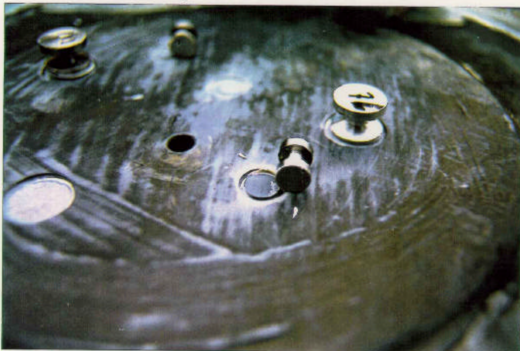
Fig. 2. Dolly testing for determination of adhesion strength.
